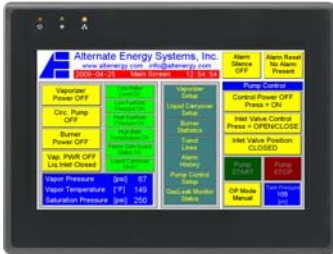
Standard EOI for Siemens S7-1200, Siemens S7-200, or Allen-Bradley MicroLogix-1100: 7-inch high-resolution (800x480) display with first-out monitor (Alarm History) 96-hour graphic TrendLine recording, trend data recording on standard SD card and remote access for monitoring and control via VNC Server / Ethernet. (unlimited client software license included).
